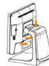
Place cables through the cable hole on the base and the top of base (original location of switch cover)
