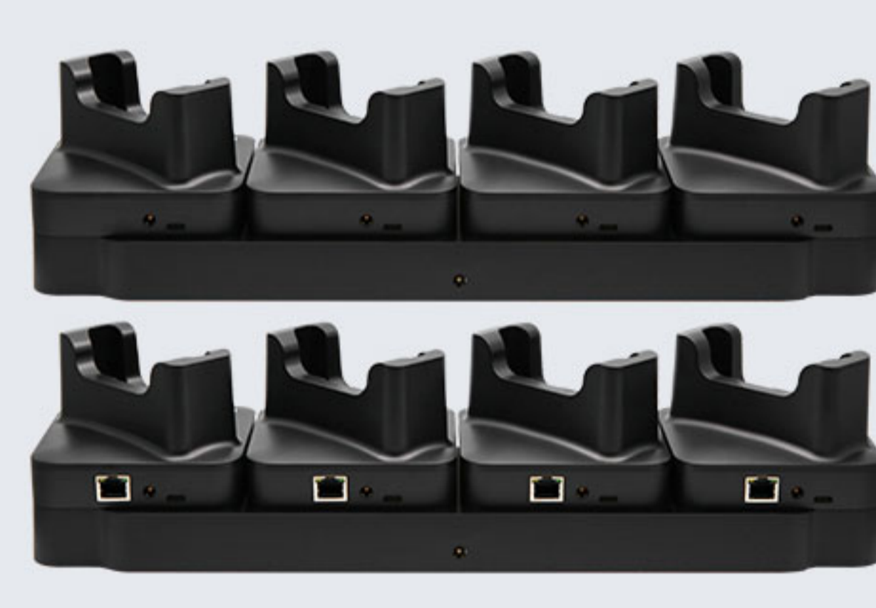
CRD-C71-RBCX4 / CRD-C71-RBCEX4 The base of 4-slots charging cradle set for any 4 pieces of cradle (CRD-C7X-DOC, CRD-C7X-DOCE, CRD-C7X-RBC, CRD-C7X-RBCE), use with DCPWR-12V2A-XX adapter.
