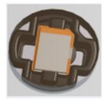
For a standard Embedded Fit 100 application, the recommended circular recess is a diameter of 14.5mm and depth of 4.5mm. Placement into the recess is carrier face down. Sourcing and validation of epoxy or potting compound used is the responsibility of the customer.
