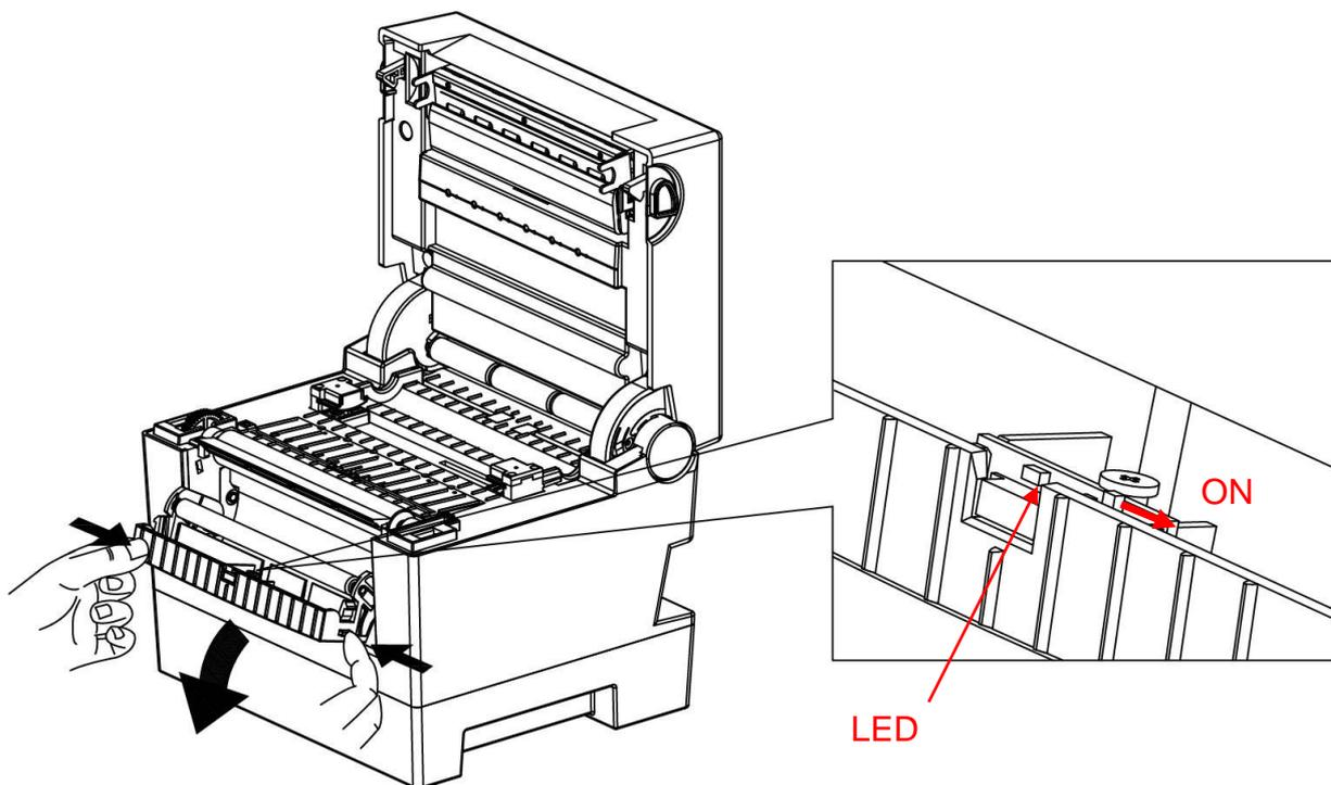
3) Remove one or two sheet of the label paper, and insert the paper as shown in the image below.
