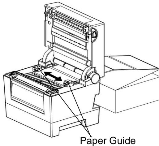
4) If you use Black-Mark or Notch paper roll, please lift up the paper and match the sensor position adjust the black mark or notch hole.
