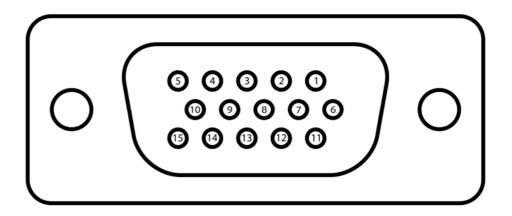
Figure 2 Pin-out of DE15 connector
