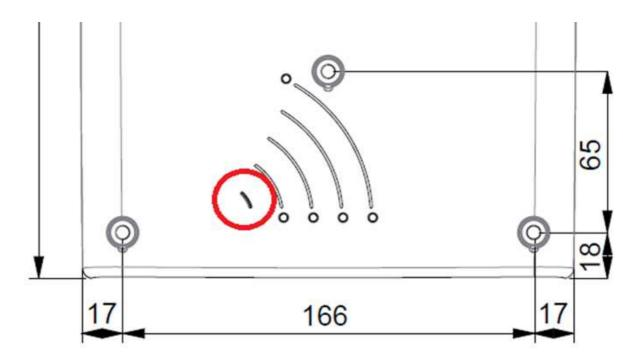
Figure 3 Location of capacitive sensor
