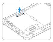
3. Install the reader using the screws provided.
