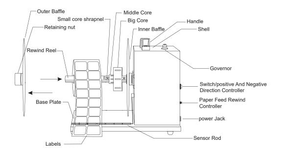
Label Rewinders, No need manual rewind when printing, Resolve trivial manual rewinding process, Reduce labour intensity, Improve label printing quality (labels stick dust easily or destroy if not rewind on time). It can help enterprises save labor cost, Promote working efficiency, Improve enterprise image, it is the good helper for the labeling personnel, Also it is the good partner for the boss.
