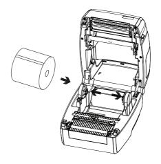
4.Pass the label through the label guides, then adjust guides to adapt to the label width.
