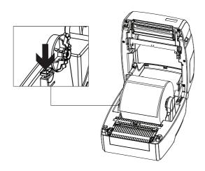
5. Press the cover lock and close the cover slightly.
