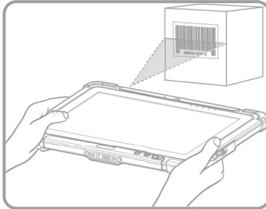
2. Press the Fn2 button. Center the aiming beam over the barcode.
