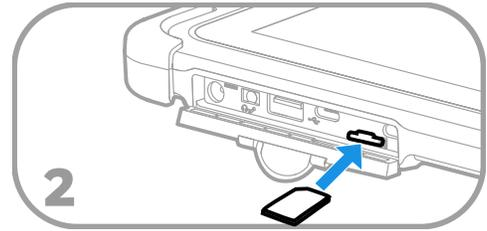
**Note:** Always power off the tablet before attempting to install or remove a card.
