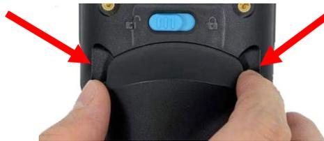
3. Pull the pull tab in the battery compartment to remove the battery. Make sure the pull tab stays inside of the battery compartment when closing the cover.
