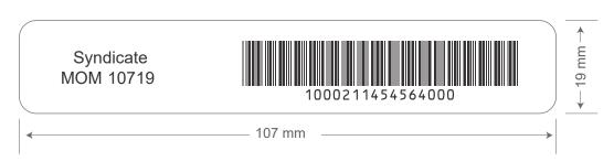
Syndicate MOM 10719 is a passive UHF RFID label for Mount on Metal applications requiring a narrow printable tag product. This product is finished with a high performance permanent adhesive for use on and off metal surfaces. These labels feature a film face to print private logos, product information, or scannable barcodes directly on the label and its additional flexibility for curved surfaces makes it perfect for tracking a variety of transit items.
