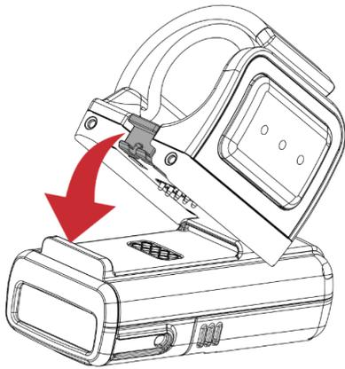
Figure 11 Trigger Assemble\_Right hand mount
