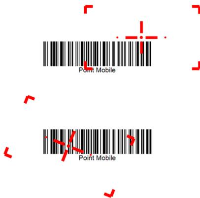
If you aim the barcode wrong direction or aim point is too tilted to scan only the part of the barcode, you can't read the barcode.
