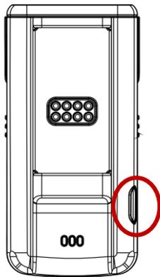
You can do the factory reset using Ring Control (Lite) app or special barcode, too. See the application's user guide to find how to perform the factory reset with the app, or see [Appendix – Factory Data Reset](#) to find special barcode.
