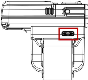
Figure 25 Sled USB connector (Open cap)
