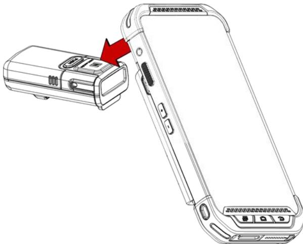
Tap-to-Pair operates like toggle in HID mode. This means that if Tap-to-Pair is performed when the ring scanner is connected to host device, the connection will be closed.
