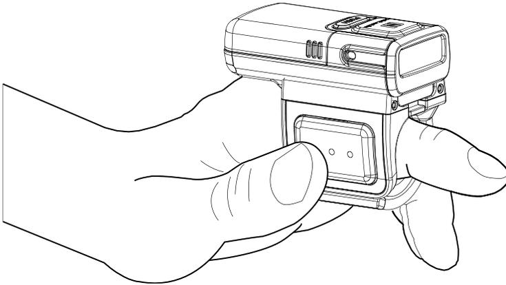
4. To loosen the finger strap, detach the end of the strap
