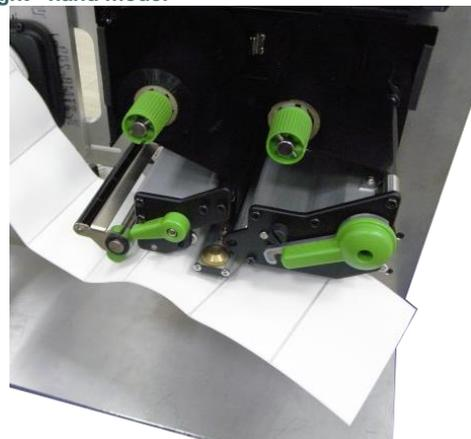
4. Adjust the rear label guide (green) to fit the label width.
