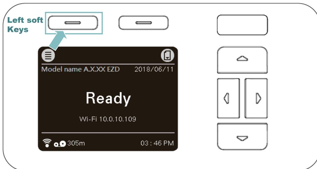
Use the navigational keys to select the "icon" (be marked in green) and press the right soft key (means
