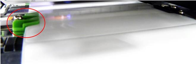
6. Move the media sensor by adjusting the media sensor position adjustment knob, make sure the gap or black mark sensor is at the location where media gap/black mark will pass through for sensing.
