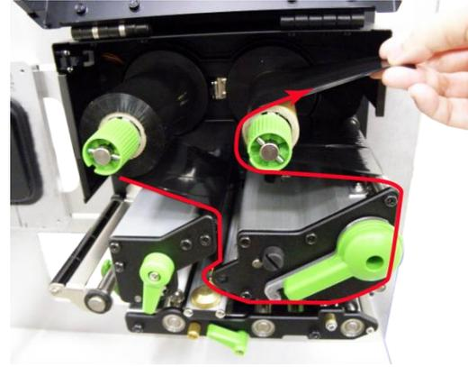
5. Wind the ribbon rewind spindle counterclockwise roughly 3~5 circles until ribbon is smooth, properly stretched and wrinkle-free.
