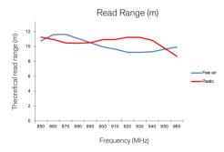
All the graphs are indicative: performance in real life applications may vary. The data has been determined based on calculations for transmitters with a 2W ERP output power level.
