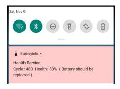
Note: If the battery is stored for the long term, it might result in accelerated battery health lower. Please try to charge and discharge your batteries several times and check the battery health is at a steady rate. If the battery health is still lower than 60%, the battery should be replaced
