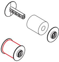
Installing small diameter of media roll
