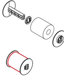
Installing large diameter of media roll
