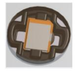
For a standard Embedded Fit 100 application, the recommended circular recess is a diameter of 14.5mm and depth of 4.5mm. Sourcing and validation of epoxy or potting compound used is the responsibility of the customer. Please see the Omni-ID Embedded Fit Tag User Guide for epoxy types qualified by Omni-ID and more information on the custom service options.
