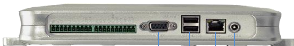
GPIO, RS485, GND, Wiegand, RS232 USB RJ45 Power
