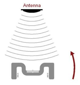
$\label{eq:angular} \begin{array}{l} \mbox{Angular Sensitivity} \\ \mbox{Inlay is rotated in the x, y, plane about the z axis} \\ \mbox{(tag shown at 0° with respect to face of antenna)} \end{array}$
