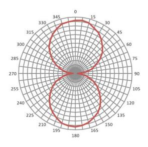
Angular Sensitivity (Relative Read Range vs. Orientation)
