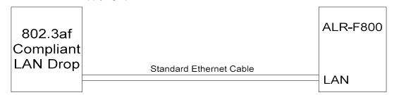
Figure 12 – 802.3af Network Connection Diagram
