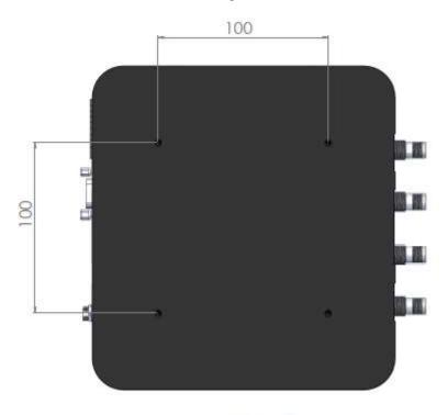
Threaded Mounting Holes (2 x 2 ; M4 Screws)
