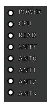
Figure 7 – ALR-F800 Front Panel Reader Diagnostic LEDs
