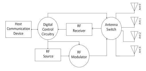
Figure 4 - System Architecture for the ALR-F800 Reader
