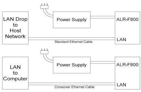
Figure 11 – 12V DC cord and Network Connection Diagram
