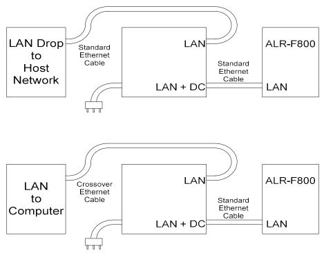
Figure 10 – PoE Power Supply and Network Connection Diagram
