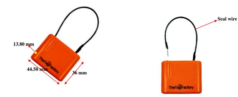
Note: Tolerance applicable are **Length:** ±1mm, **Width:** ±0.5mm and **Thickness:** ±0.3mm
