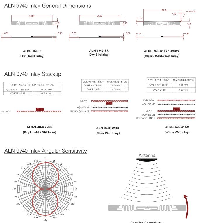
Angular Sensitivity (Relative Read Range vs. Orientation)
