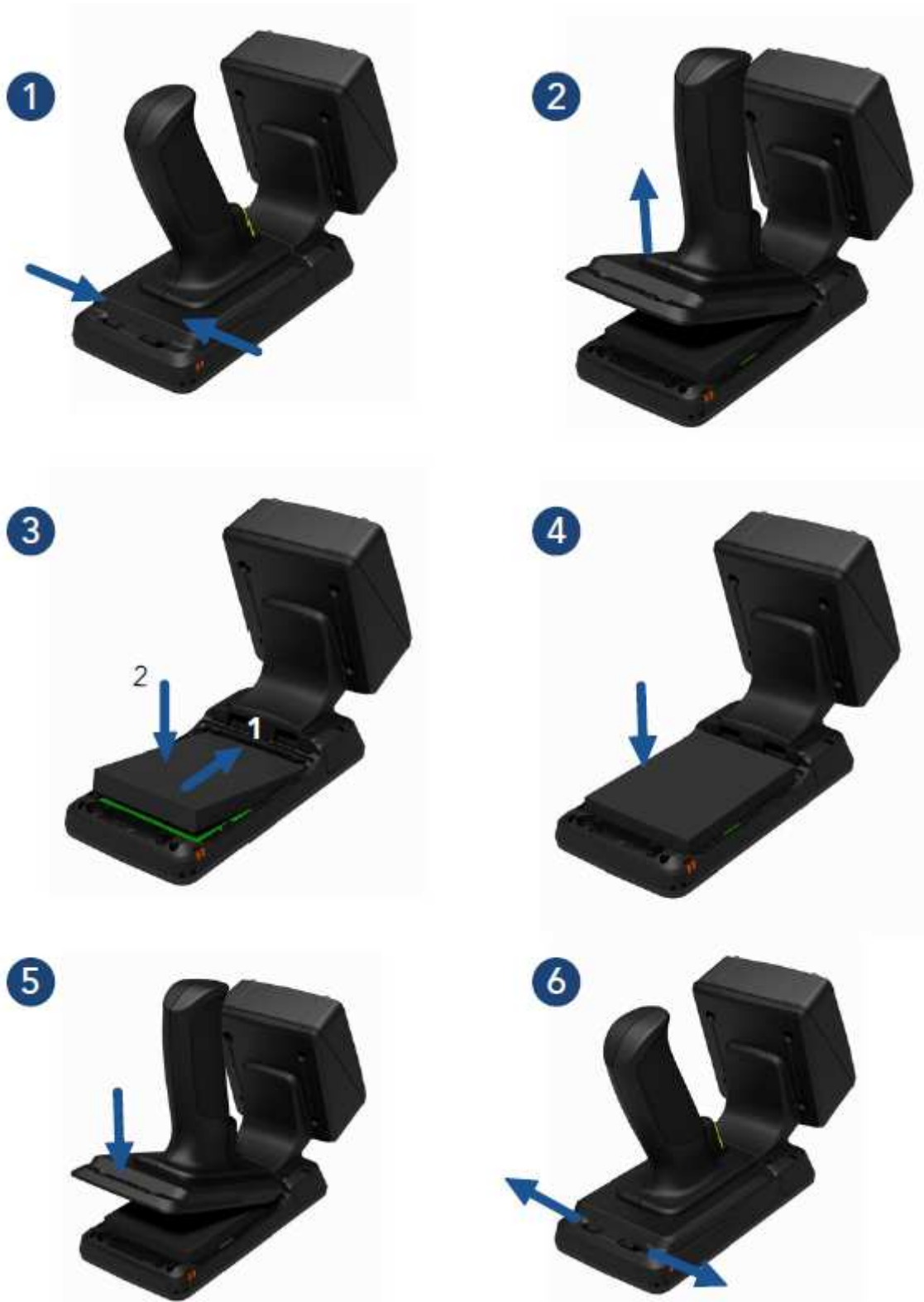
Picture 2 Installing battery
