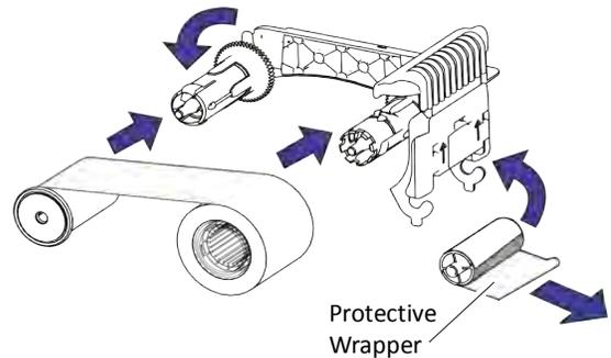
3. Load the cleaning roller on the ribbon cartridge.
