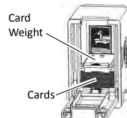
7. Close the cartridge door. This releases the card weight so that it is lowered on top of the cards.
