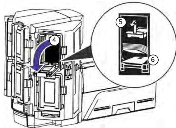
6. Load the cards into the input hopper cartridge. Handle the cards by the edges only, or wear approved card inspection gloves.
