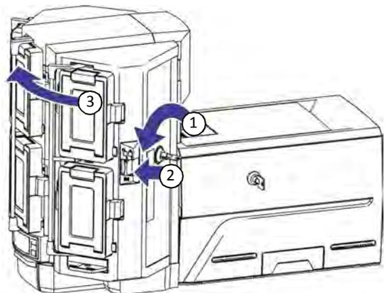
4. Press the cartridge release button at the top of the cartridge and open the cartridge door.
