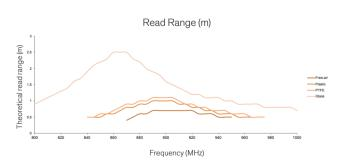
Read range with Impinj Mini-Guardrail antenna, 1W transmission power
