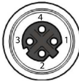
Figure 2 - M12 D-Coded Female Ethernet Network Connector
