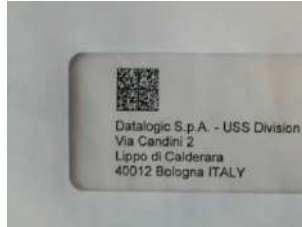
Figure 16 - Address Coded in Data Matrix Symbology for Automated Mail Processing
